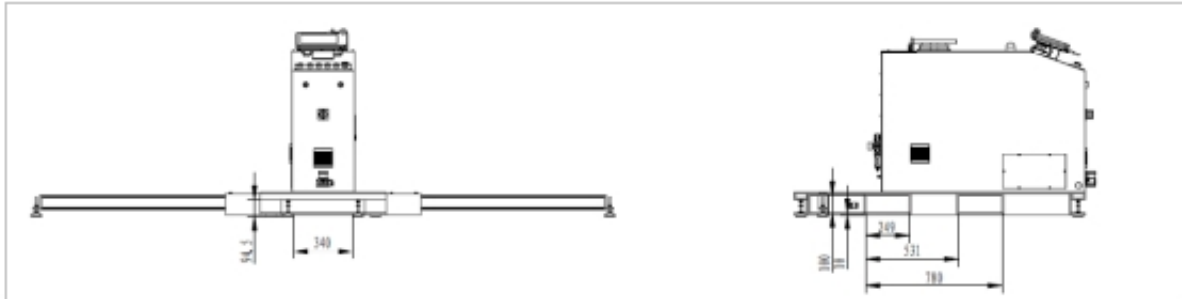
Figure 4.15 Alignment of slots and bases and corresponding dimensions
